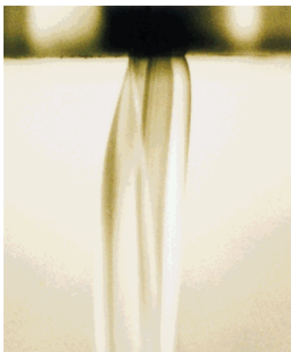
Figure 11 Melt-twist behavior of PP via spinnerette C at 220°C. [Color figure can be viewed in the online issue, which is available at www.interscience.wiley.com .]
